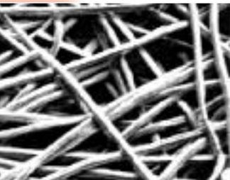
*Micron-level metallic fibers are key to the exceptional performance of Fibermet and PMF media.*
